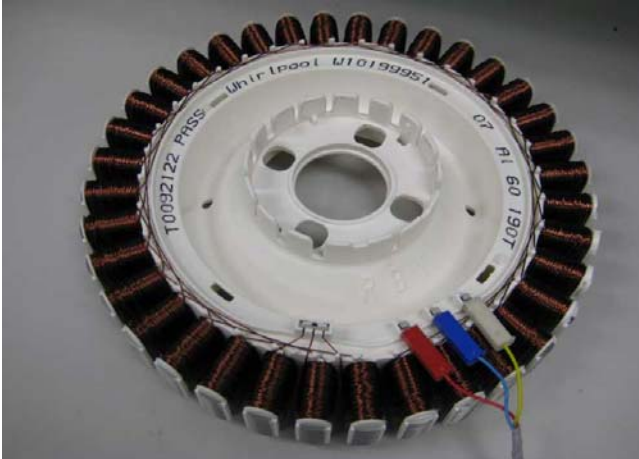
Aluminium Stator (36 Poles)
